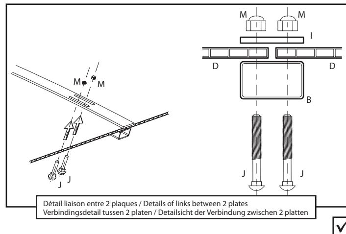
Détail liaison entre 2 plaques / Details of links between 2 plates
